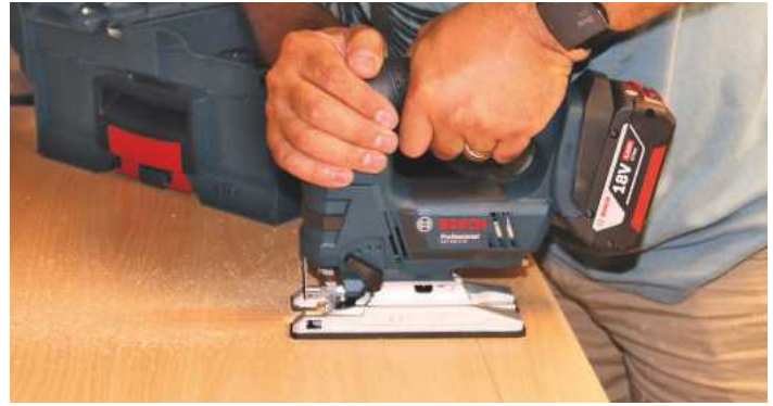
▲ Once it has pierced the work you can cut as normal
